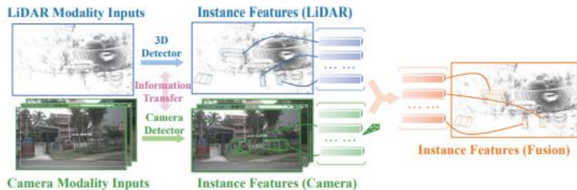
(c) Overview of our sparse fusion strategy. We extract instance-level features from the LiDAR and camera modalities separately, and fuse them in a unified 3D space to perform detection.
